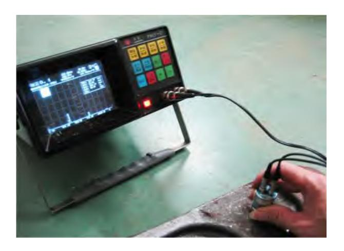
Ultrasonic Testing Machine (A)
