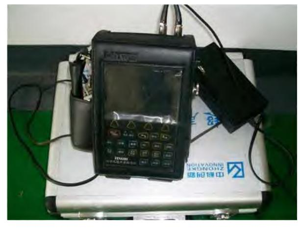
Ultrasonic Testing Machine (B)
