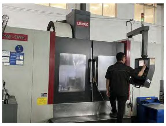
Machining Center (VMC168GL)
