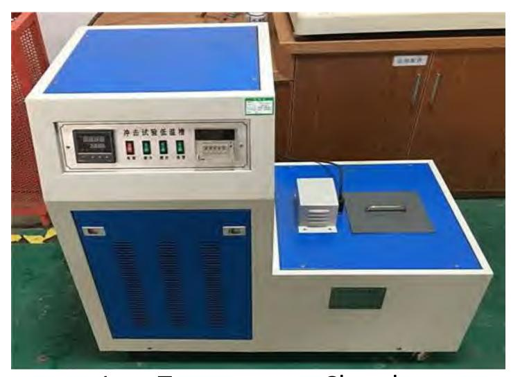
Low Temperature Chamber for Impact Specimen
