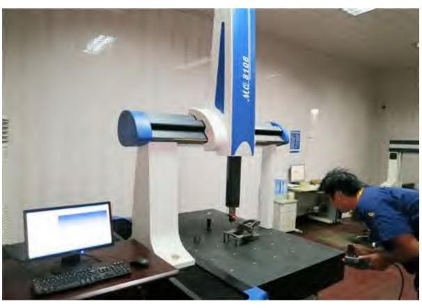
Coordinate Measuring Machine (B)
