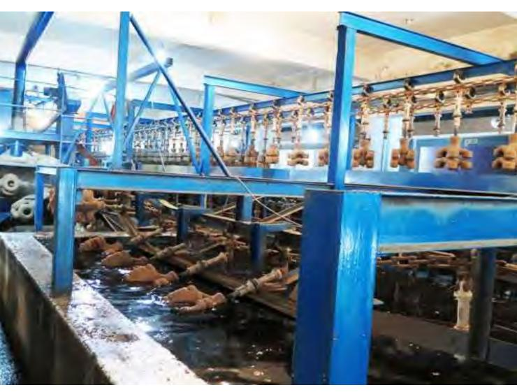
Automated Shell Making Production Line (Water Glass) A
