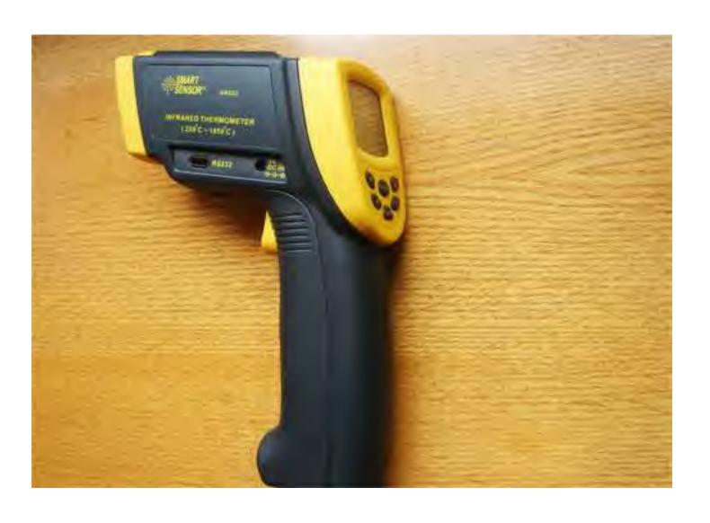
Non-contact Infrared Thermometer
