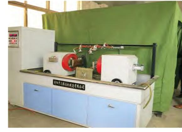
Magnetic Particle Testing
