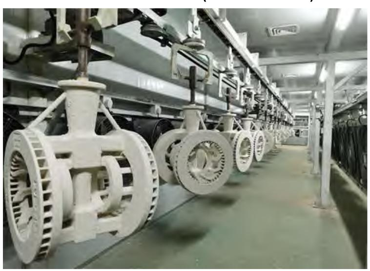
Automated Shell Making Production Line (Silica Sol) B
