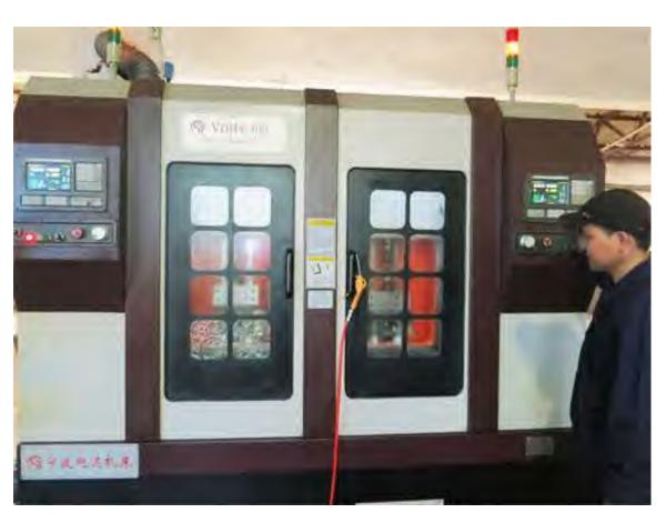
Four-station Deep Hole Drilling Machine (VDH4-300)
