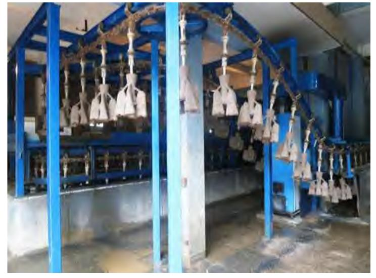
Automated Shell Making Production Line (Water Glass) B
