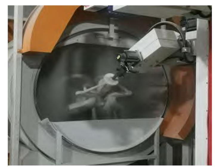
Automated Shell Making Production Line (Silica Sol) A
