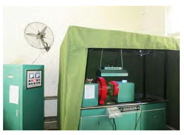
Magnetic Particle Testing
